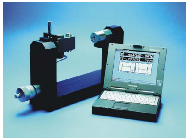
L-700 Twin Barrel Extruder Alignment System
